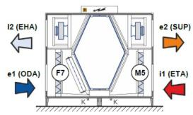
Install air filters before putting the unit into service to avoid contamination.
